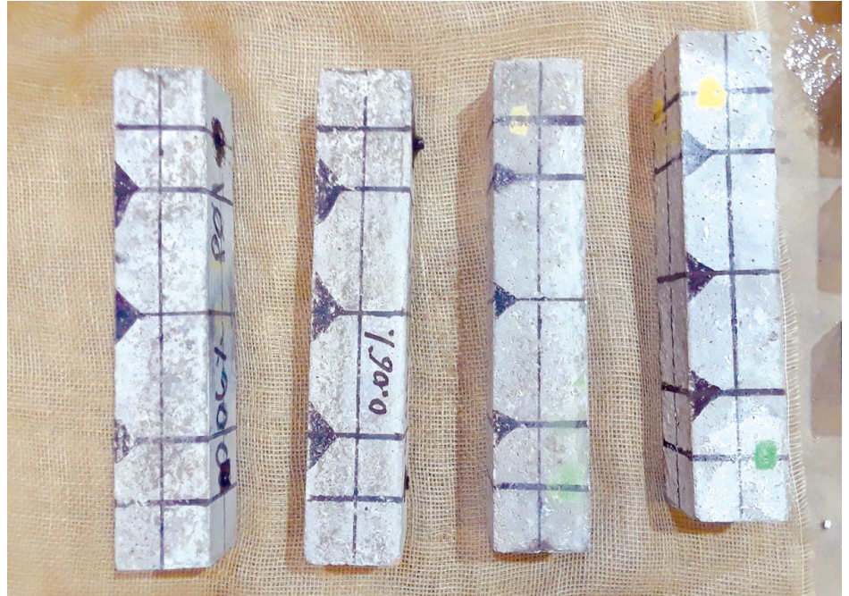
Biomimetic Antifreeze Polymer-Modified Concrete sample that passed ASTM C666, the standard test method for rapid freezing and thawing of concrete. Courtesy of the University of Colorado Boulder, College of Engineering and Applied Science.
